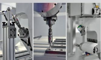
By a 3D measuring pin (option) the machine geometry is checked at a reference bolt in the machine table. In case the geometry deviates to a certain extent, an error message is shown at the control. This guarantees a quick adjustment of the machine, for example after a crash or in order to improve quality.
