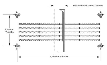
A centre partition is provided for independent machining in area 1 and area 2. The centre partition is moveable by 500mm in X-direction. Hereby the working area is extended by 250mm in X-direction. The free inserting width is reduced by 250mm in the opposite station. The centre partition only moves with a change of station.
