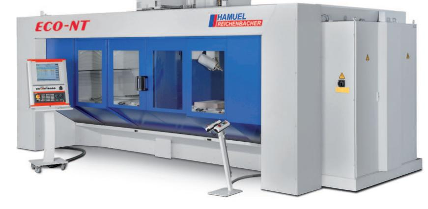
Depending on the application also a chain magazine with 40 places or other special versions are possible. The high performance frequency spindle with up to 60,000rpm, the blast nozzle (with air ionization to
