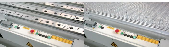
The open tubular frame has a surface loading of up to 1,000kg. The supporting beams are mounted in a grid of 200mm in Y-direction and equipped with threads and setting bushes in a grid of 100mm in X-direction.
