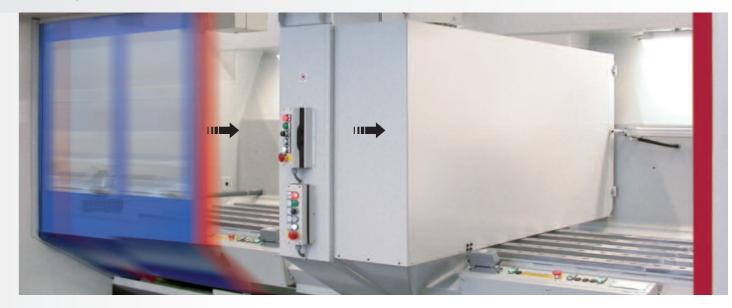
The loading area is shut by two motor-driven sliding doors (option). With reciprocal loading each door can be opened individually. A centre partition between the working areas provides protection against flying parts from the opposite working area. Alongside the tables chips fall onto the machine bed. The construction of the sheet metal coverings prevents the formation of chip clusters.
